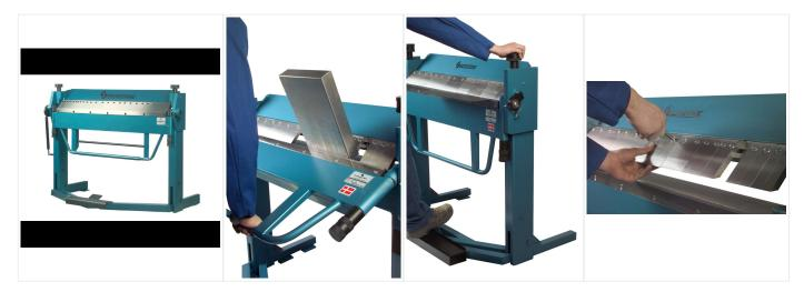
The SCANTOOL SCAN 13S is manufactured with a segmented upper beam and a foot operated upper beam to allow simple and fast hands-free operation.
