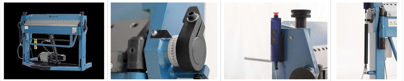
The SCANTOOL SCAN 10S & 13S are actually manual machines, which have been up-rated to offer a very efficient motorised option via a developed and patented, folding beam support cylinder system.
