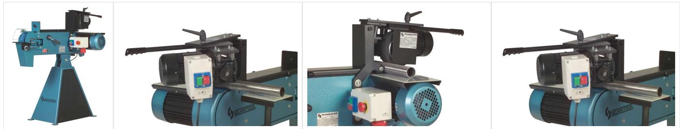
Scantool 75 CG centerless grinding and polishing machines are supplied with an attachment which can be mounted on all belt grinders with a 75x2000 mm belt and with a large grinding surface on top.
