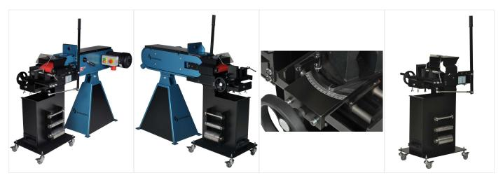
Scantool 150RB is, first and foremost, a pipe notcher which grind pipes of all types (round, square, solid) and with diameters of between 17 mm and 100 mm.
